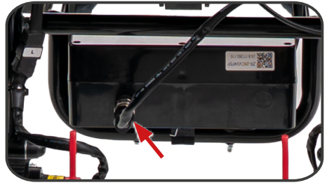
Illustration 8. Connecting the battery power connector.
