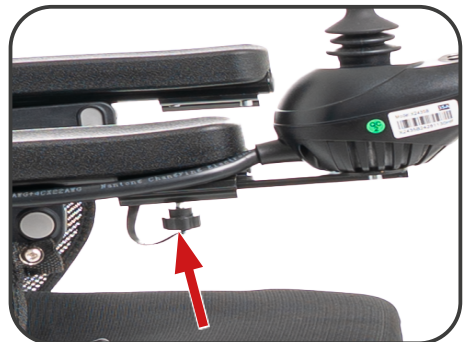
Illustration 12. Control panel adjustment screw.
